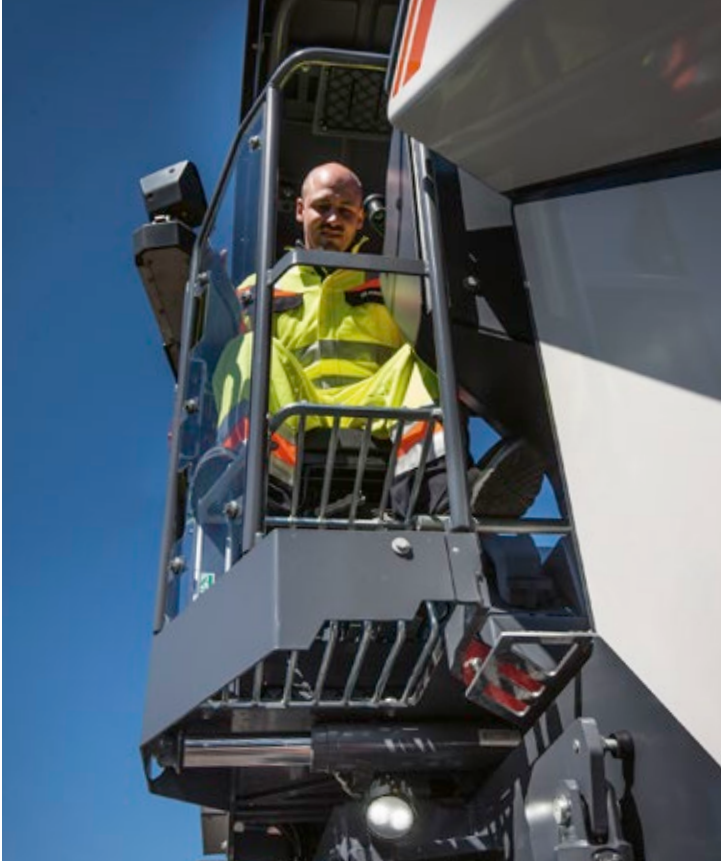
The movable operator's platform provides an ideal overview of all important working areas.
