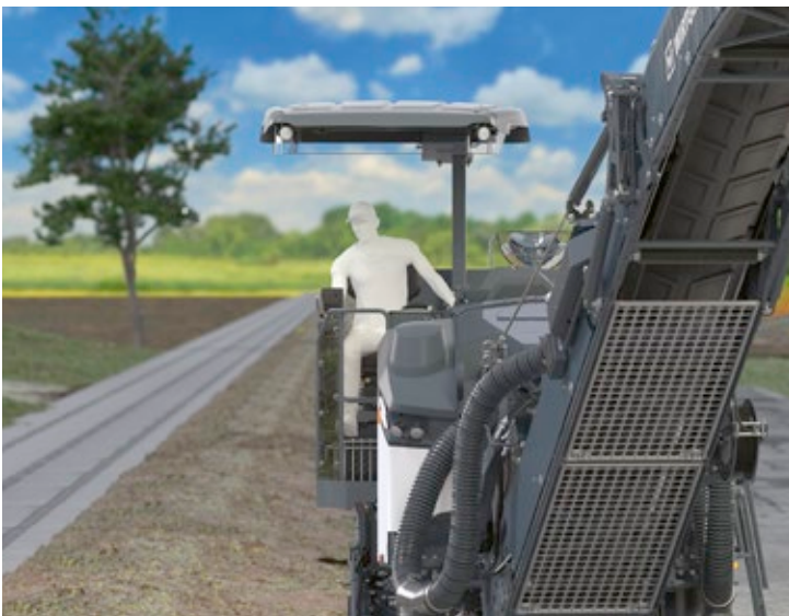
The vertically and horizontally adjustable weather canopy provides optimum protection in a range of different working positions - especially on construction sites with restricted space.
