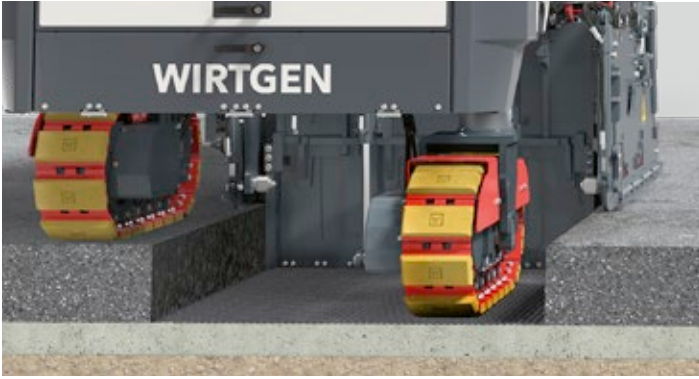
Milling drum assembly FB1500 (4 ft 11 in) with Multiple Cutting System MCS BASIC .
