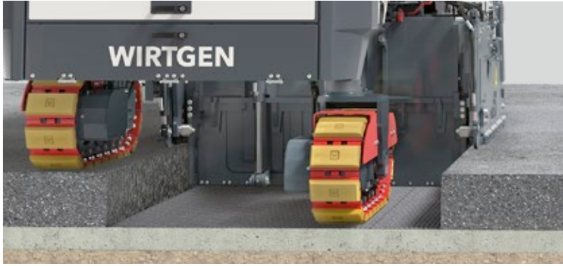
Milling drum assembly FB1800 (5 ft 11 in) with Multiple Cutting System MCS BASIC .
