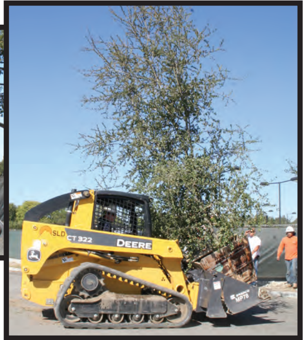
(Above) Vice President of Sierra Landscape, Kevin Watchler. (Right) The John Deere CT322 compact track loader placing tree boxes.
