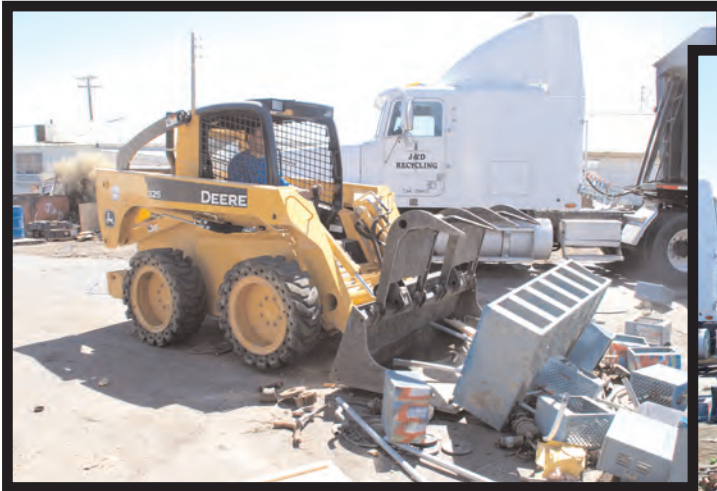
(Above) J&D Recycling's John Deere 325 skid steer pushes the scrap material into piles for easier pick-up. (Above Right) The JD 50D ZTS compact excavator processing a load of scrap.
