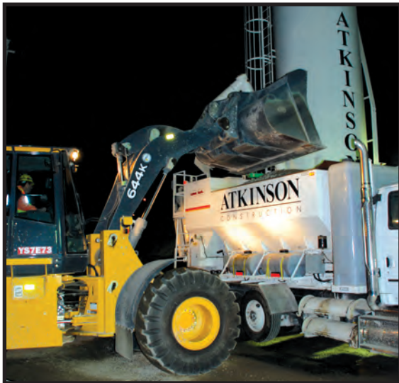
(Left & Above) Atkinson Construction's JD 644K Wheel Loader purchased from Coastline Equipment Co. loading a volumetric truck for work on the I-10 Freeway Rehabilitation Project.
